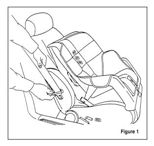
3. While holding the shoulder and lap belt portions together, route the tongue through the child seat according to the child seat manufacturer's instructions. See Figure 2. Be sure that the belt webbing is not twisted.
